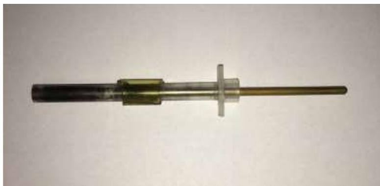
**Figure 2.** Carbon paste electrode after done.
